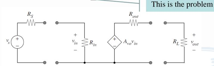
... but excellent transconductance amplifier (want high  $R_{in}$ , high  $G_{mo}$ , high  $R_{out}$ ):  $G_{mo} = g_m$
