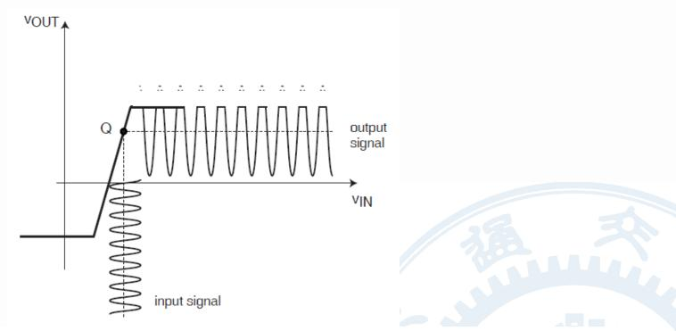
•Transfer characteristics linear over limited range of voltages: amplifier saturation.
