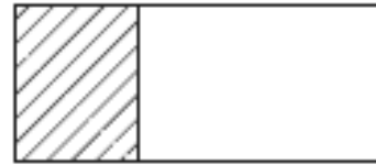
Asymmetrical inductive diaphragm
