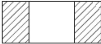
Symmetrical inductive diaphragm
